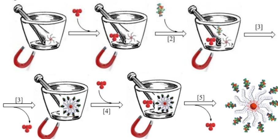
[1] solubilization of core/shell nanosystem in chloroform; [2] essential oil added drop by drop; [3,5] mixing until evaporation the chloroform; [4] chloroform added drop by drop.
