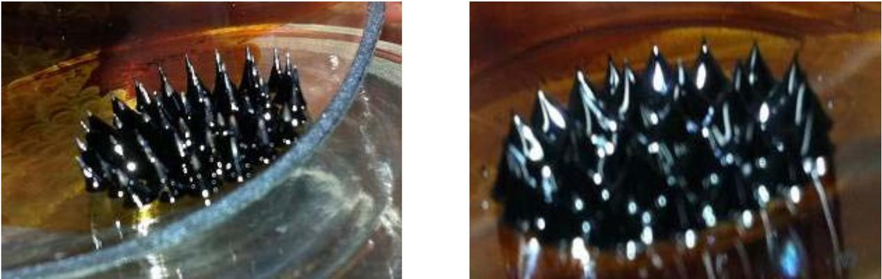
**Figure 3.** Magnetic field aligns the core/shell/extra-shell nanofluid
