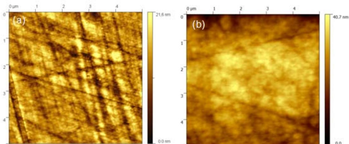
**Figure 2.** Topographic tapping AFM images of bare glassy carbon electrode (a) and Poly-Lysine/Au NP 500/dsDNA film modified glassy carbon electrode (b)
