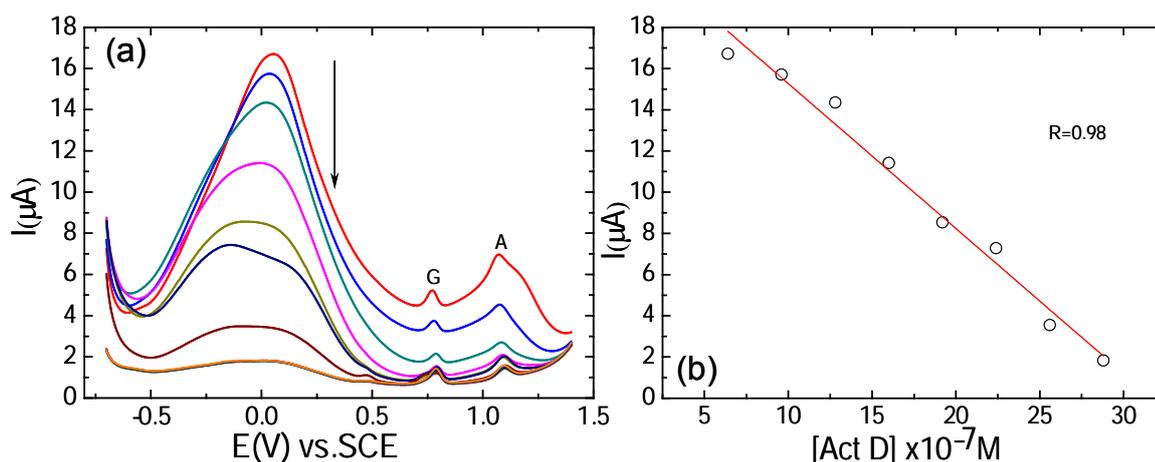
**Figure 5.**(a)Differential pulse voltammograms recorded at the pLys/AuNP500/dsDNA/ssDNA modified GC electrode in acetate buffer solution containing 53μg/mL single stranded DNA and Actinomycin D of  $3.2 \times 10^{-7} \text{M}$  to  $29 \times 10^{-7} \text{M}$ .(b)Variation of peak current at 0.05V with increasing concentration of ActD.
