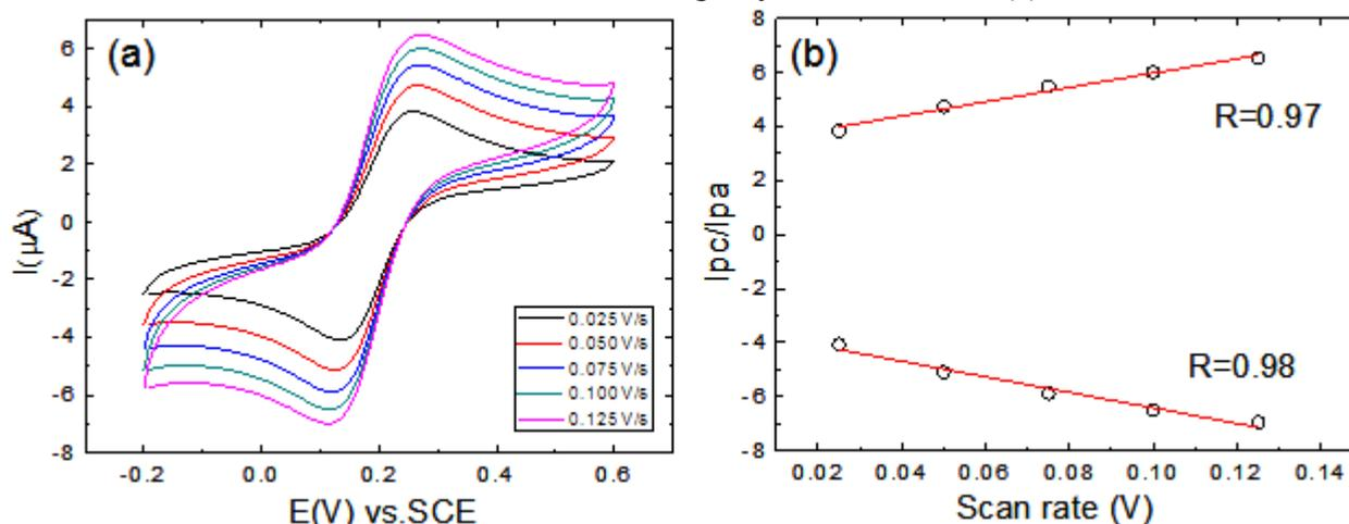
**Figure 3.**(a). Cyclic voltammograms recorded at the pLys/AuNP500/dsDNA modified electrode in aqueous solution of 0.0005M  $[\text{Fe}(\text{CN})_6]^{3-/4-}$  and 0.1M  $\text{NaClO}_4$  at increasing scan rates (see inset).(b)Linear variation of anodic and cathodic peak currents with increasing scan rates.
