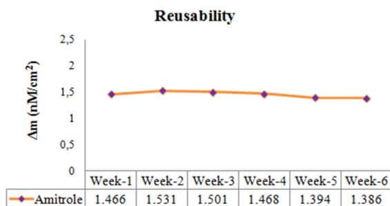
Fig. 6. Reusability of amitrole imprinted QCM sensor.
