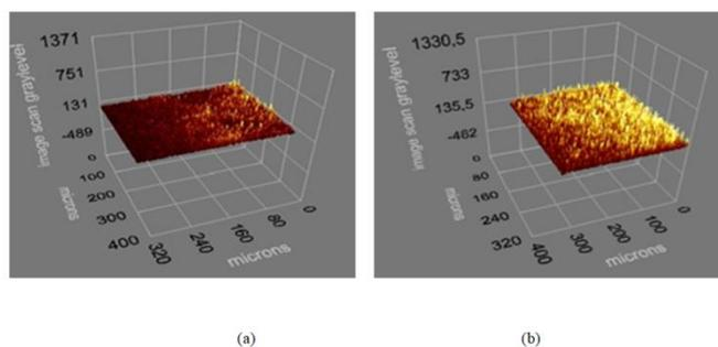
Fig. 2. Ellipsometer images of a) nonimprinted and b) Amitrole imprinted QCM sensor surfaces.
