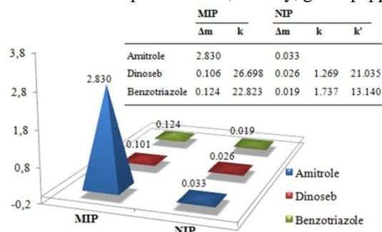
Fig. 5. The selectivity comparison studies of amitrole imprinted sensor with dinoseb and benztiazazole.
