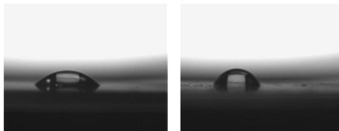
Fig. 3. Contact angle measurements of a) nonimprinted and b) Amitrole imprinted QCM sensor surfaces.
