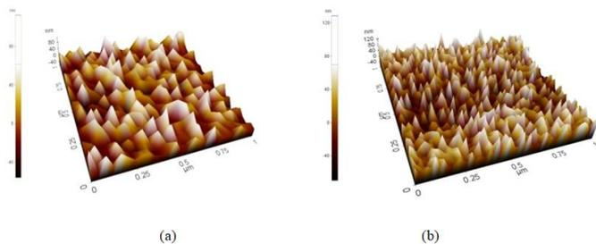
Fig. 1. The atomic force microscopy images of a) nonimprinted and b) Amitrole imprinted QCM sensor surfaces.
