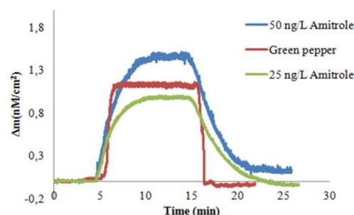
Fig. 7. Amitrole analysis in green pepper by amitrole imprinted QCM sensor.
