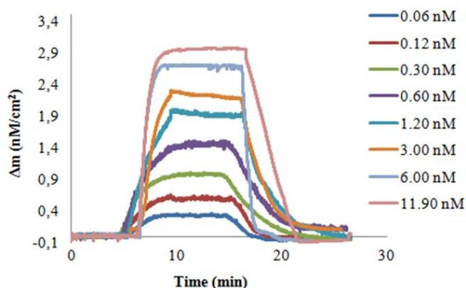
Fig. 4. The real-time Amitrole detection chart (Mass (nM/cm<sup>2</sup>)-Time) by Amitrole imprinted QCM sensor at different concentrations.
