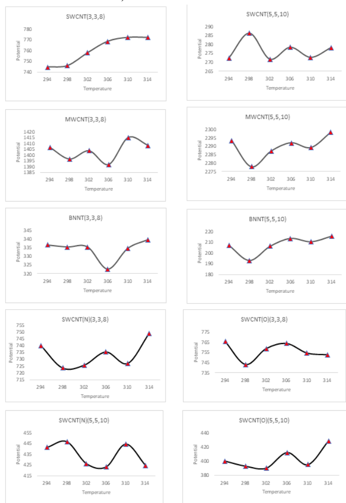
Figure 1. The lowest potential energy of Nanotubes+ H 2 O by Monte-Carlo simulation using OPLS method at 294-314 K.
