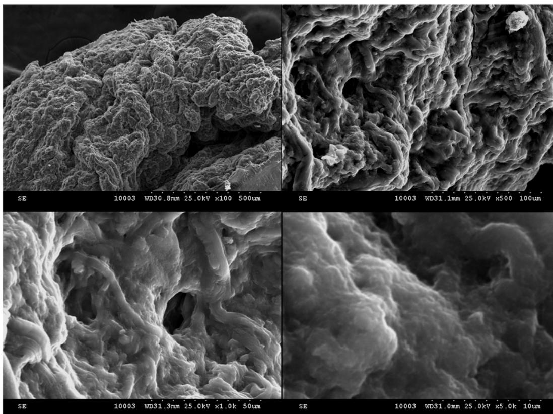
**Figure 4:** SEM micrographs of fabricated water soluble biocomposite
