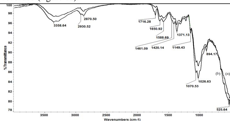
**Figure 2:** FT-IR spectra of chitosan (a) and fabricated water soluble biocomposite (b)
