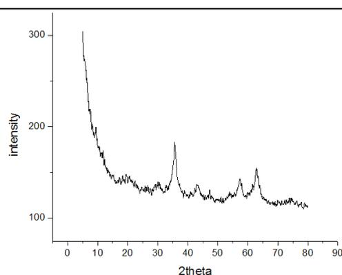
**Figure 3:** XRD pattern of fabricated water soluble biocomposite
