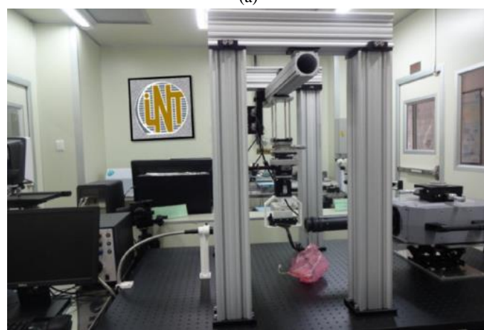
Figure6. (a) General Schematic of Electrostatic inkjet printing With Forces acting on the ink at the tip of the nozzle (b) Real setup of the optical bench at INT for characterisation and simulation of the inkjet process
