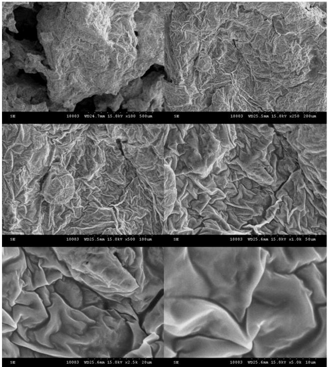
Figure 2: SEM micrograph of CHT/ALG composite
