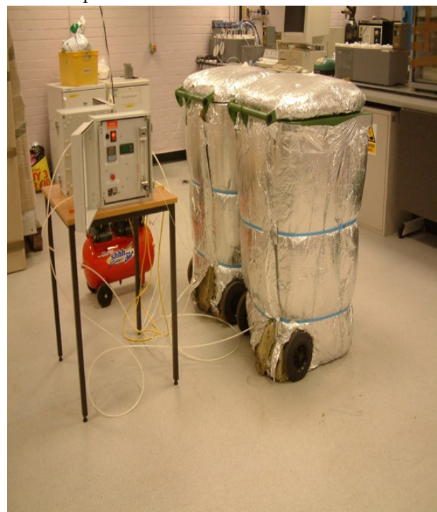
Picture 1. Bin used for composting trial, with air supply system.
