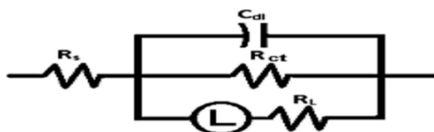
Figure 4. Equivalent circuit applied to fit the impedance outcomes.
