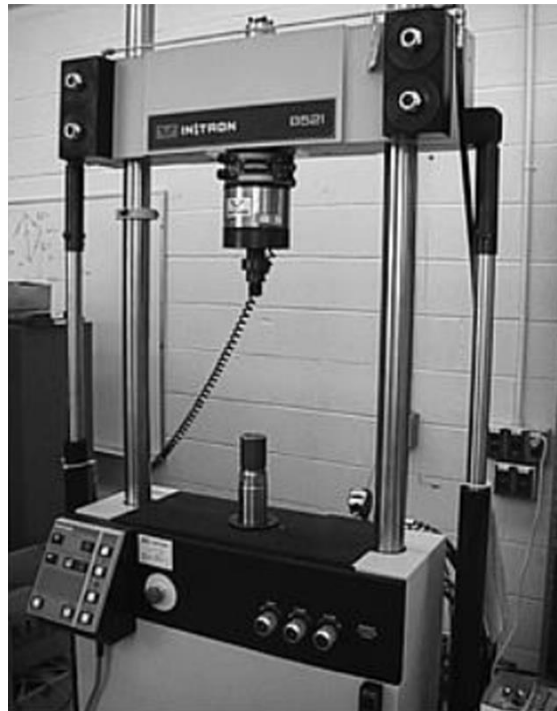
Figure 3. Fatigue Testing Machine (Instron, Model 8801, United States).
