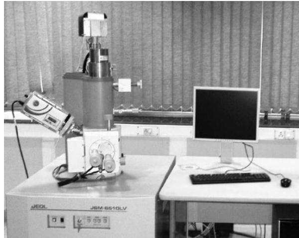
Figure 1. Scanning Electron Microscope used for microstructure analysis (JEOL, Model JSM 6510LV, Japan).
