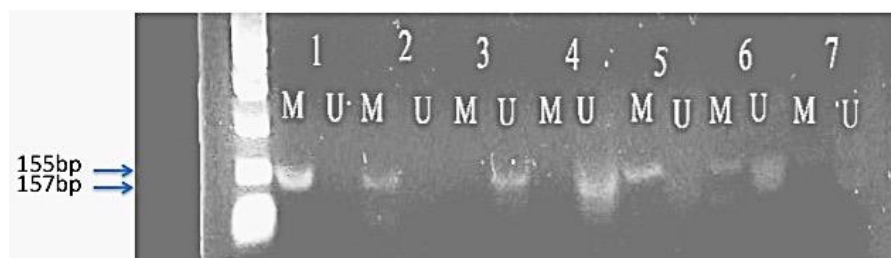
Figure 4. Fig. 3 "In situ" BRCA2 promoter methylation (amplicon 155pb-M; 157pb-U). Methylated DNA samples for BRCA2 gene promoter are 1,2,5,6. The unmethylated samples: 3,4,6, while the sample nr. 6 presented both methylated and unmethylated alleles.
