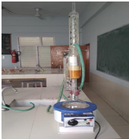
Figure 1. Extraction of plant leaves extracts using soxhlet extractor unit.
