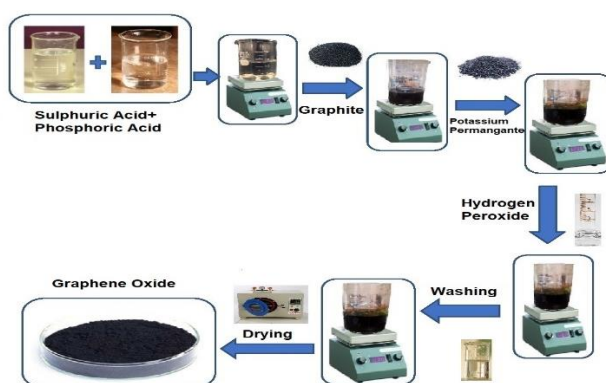
Figure 1. Schematic representation of the synthesis of graphene oxide.
