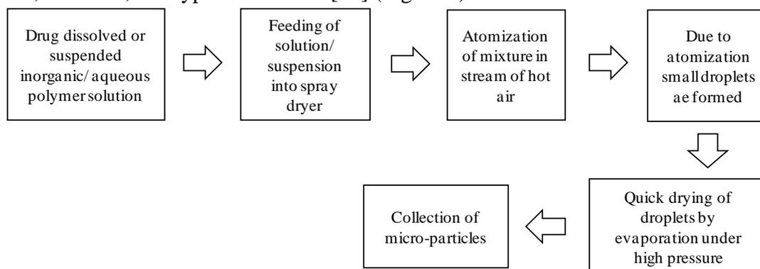
**Figure 6.** Spray drying technique for microparticles production.
