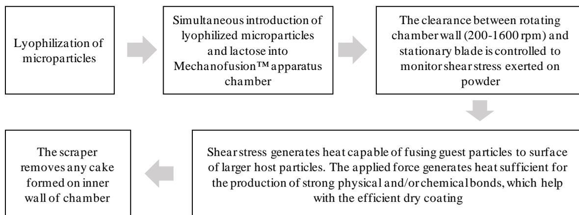
**Figure 4.** Dry coating technique for microparticles production.
