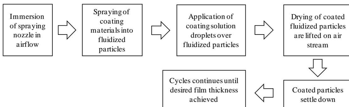
**Figure 5.** Air suspension technique for microparticles production.
