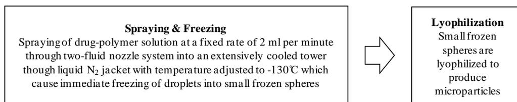
**Figure 7.** Spray freeze-drying technique for microparticles production.
