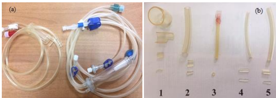
Figure 1. a) Arterial and venous dialysis blood tubings, b) Types of dialysis tubings with different wall thicknesses, 1) 1.8 mm, 2) 1.5 mm, 3) 1.3 mm, 4) 1.2 mm, 5) 0.5 mm and their corresponding parts tested.
