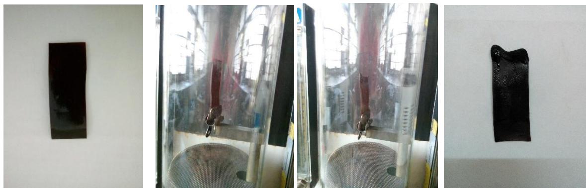
Figure 10. LOI test performance (a) FWBPU film sample; (b) Sample kept in the LOI testing apparatus before the analysis; (c) After completion of LOI test; (d) sample removed from the LOI testing apparatus.
