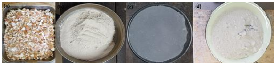
Figure 1. Particulate reinforcements (a) Sourced eggshells; (b) Milled eggshells; (c) Carbonized eggshells at 800°C; (d) Fly ash.
