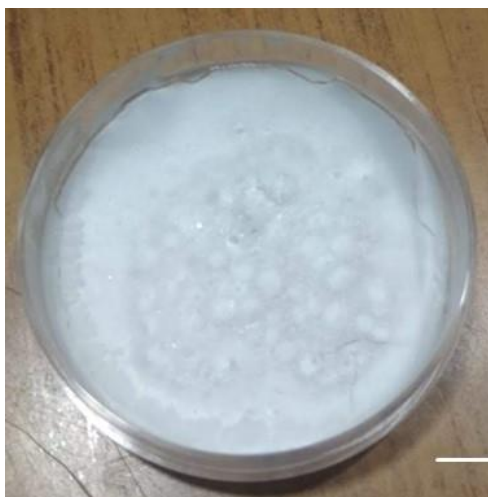
Figure 1. The lyophilized form of GelMA synthesized using 20% methacrylic anhydride. The scale bar is 3 cm.
