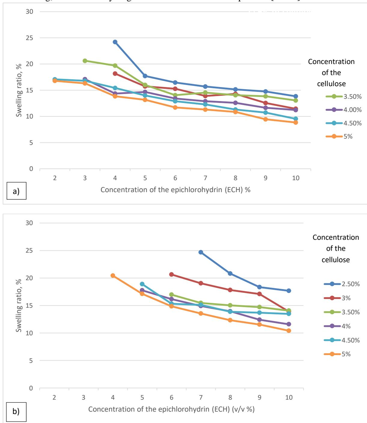
**Figure 5.** The experimental data of swelling ratio of cellulose hydrogel (a) by the freezing method and (b) by the heating method.
