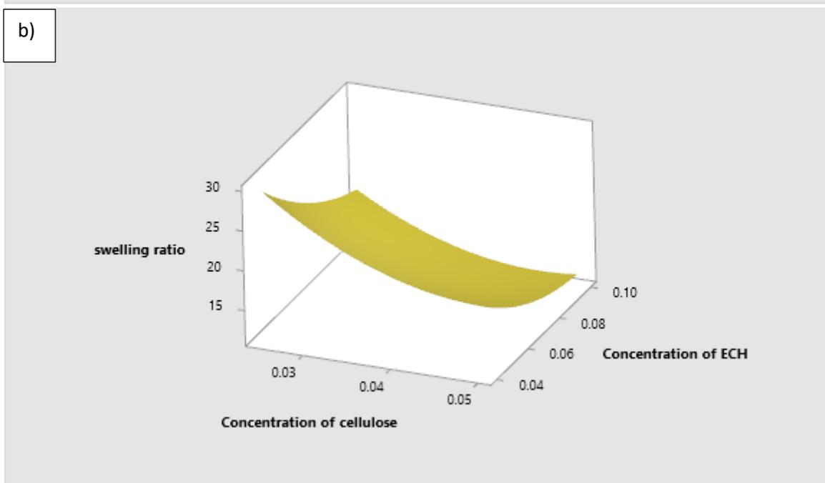
**Figure 4.** The surface plots of the swelling ratio versus the concentration of cellulose and ECH (a) by the freezing method and (b) by the heating method.
