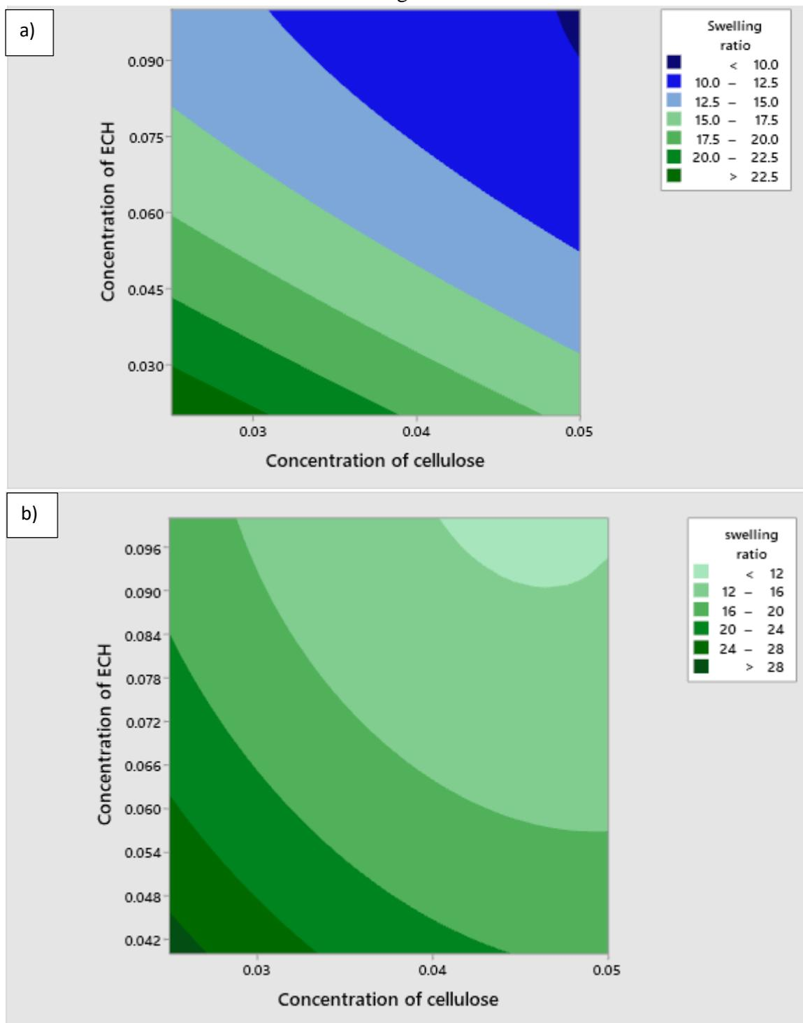
**Figure 2.** The contour plots of the swelling ratio of the cellulose hydrogels by (a) freezing method and (b) heating method.
