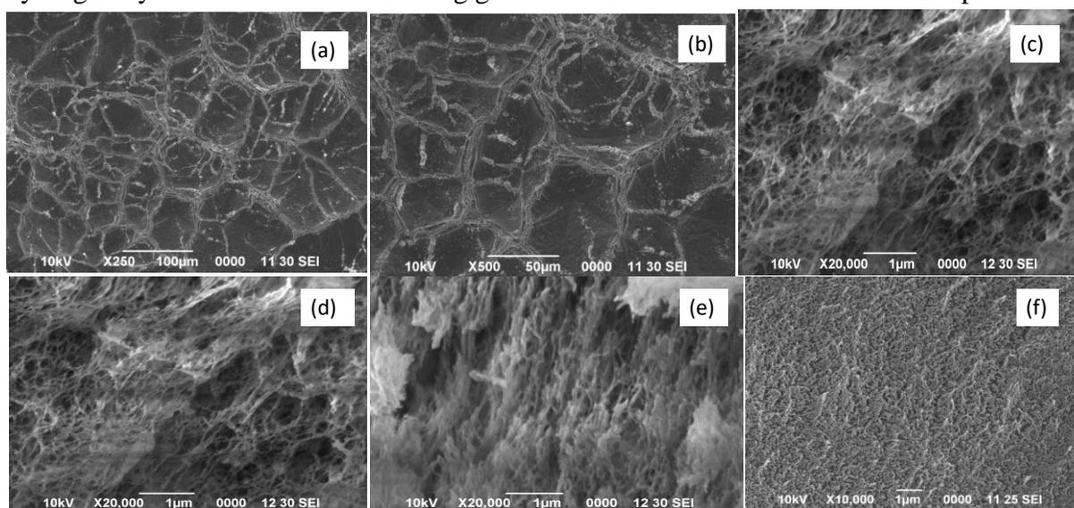
**Figure 1.** SEM images of cellulose hydrogel synthesized with (a) 3 (w/v%), (b) 4 (w/v %), (c) 5 (w/v%) of cellulose solution under heating method; (d) 3 (w/v%), (e) 4 (w/v %), (f) 5 (w/v %) of cellulose solution under freezing method with 3 % of ECH as a crosslinker
