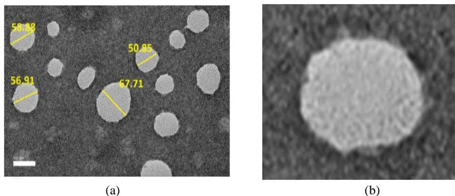
**Figure 5.** Transmission electron microscopy (TEM) images of the formulated nanoemulsion containing crude extract of *C.asiatica* (a) on the scale of 50 nm, and (b) magnified spherical shape.
