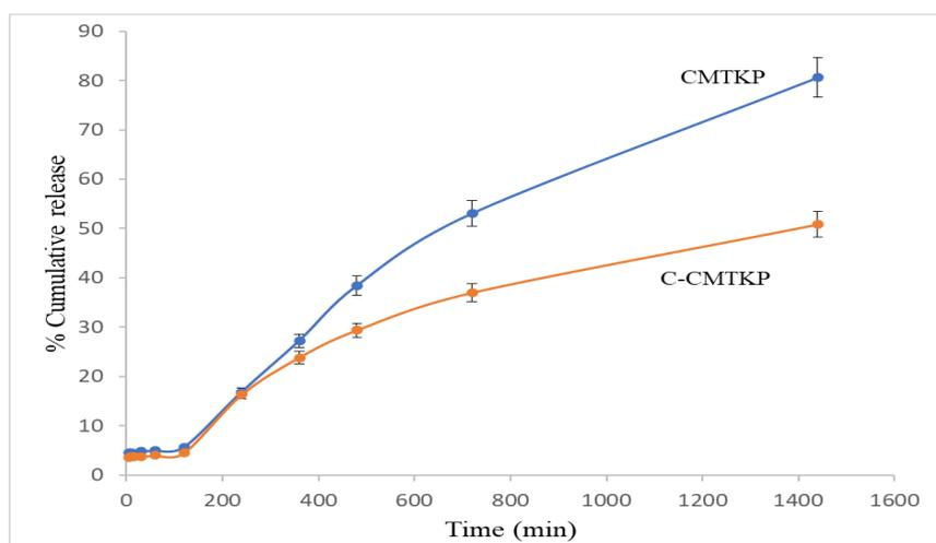
**Figure 7.** The drug release profile of diclofenac sodium tablet composed of CMTKP and C-CMTKP.
