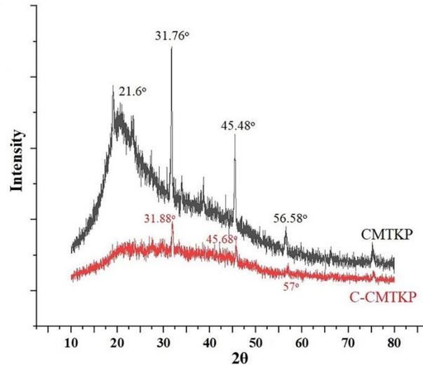
**Figure 5.** X-ray diffraction of CMTKP and C-CMTKP.
