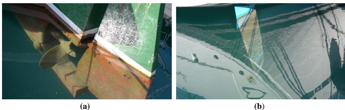
Figure 1. Marine biofouling examples (a) on a boat propeller; (b) on a rudder blade surface.
