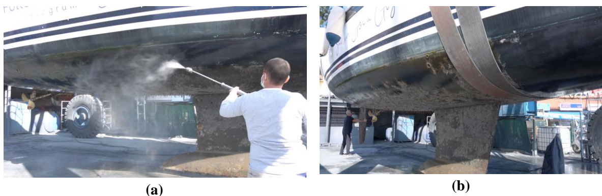
Figure 5. Example of (a) cleaning with high-pressure water, which is one of the physical cleaning methods; (b) bottom of the sailboat after cleaning process.
