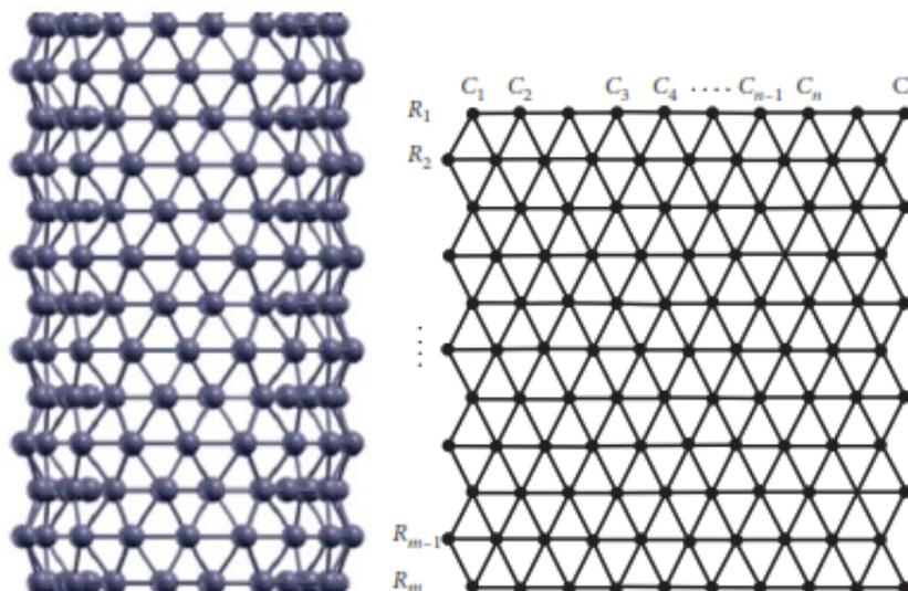
**Figure 5.** Graphical structure of Tri-Angular boron nanotube.
