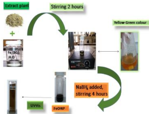
Figure 1. Preparation procedure of iron nanoparticles using an extract of Teucrium apollinis added to the ferric sulfate solution with NaBH 4 as a reducing agent.
