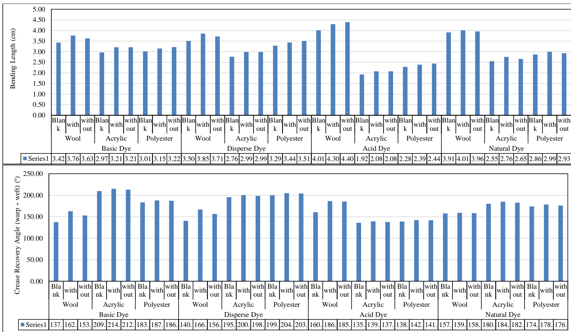
Figure 11. Bending length and crease recovery angle of different treated dyed fabrics using a different dyes nature in the presence and absence of crosslinker.
