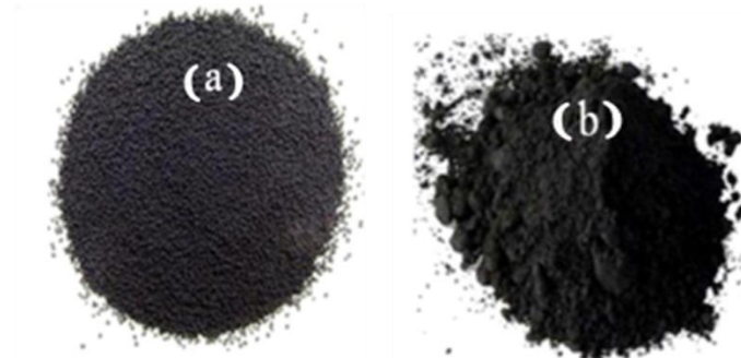
Figure3. Carbon black (CB) powder of OPP: (a) crystalline structure and (b) amorphous.
