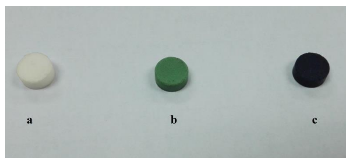
Figure 18. Images of spinels sintered at 1500^\circ\text{C} prepared using LDHs (a) pure spinel, (b) doped with 30% Ni and (c) doped with 30% Co.
