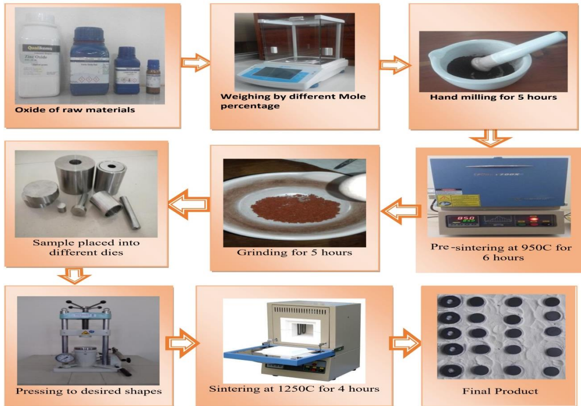
Figure 1. Flow chart of rare-earth ferrite sample preparation technique by the usual ceramic method.
