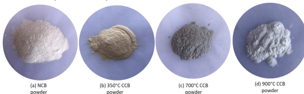
Figure 2. Calcination of cuttlefish bone at different temperatures.
