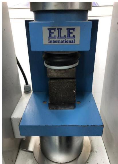
Figure 3. Testing of RHA geopolymer cube test objects using a compressive strength machine.
