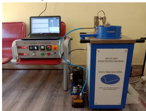
Figure 3. Pin-on-disc (POD) apparatus set up.
