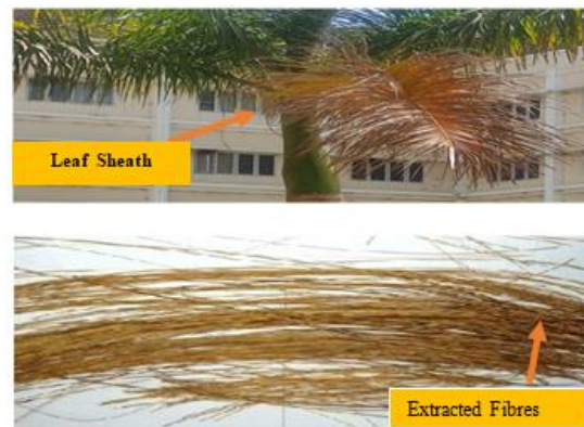
Figure 1. Extracted Roystonea regia fibres from the royal palm tree.
