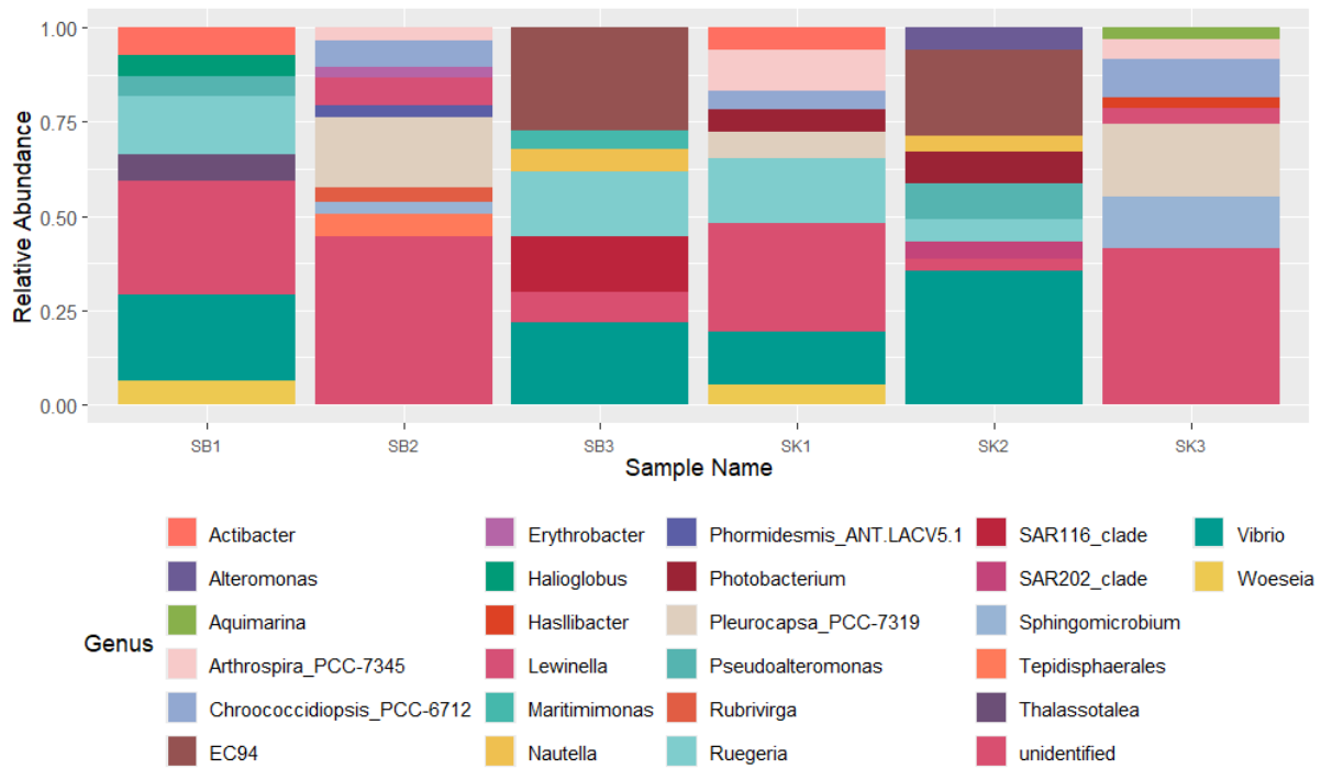
Figure 4. Genus-level bacteria composition in cement concrete (SB) and wood (SK) material surface with 2% abundance.
