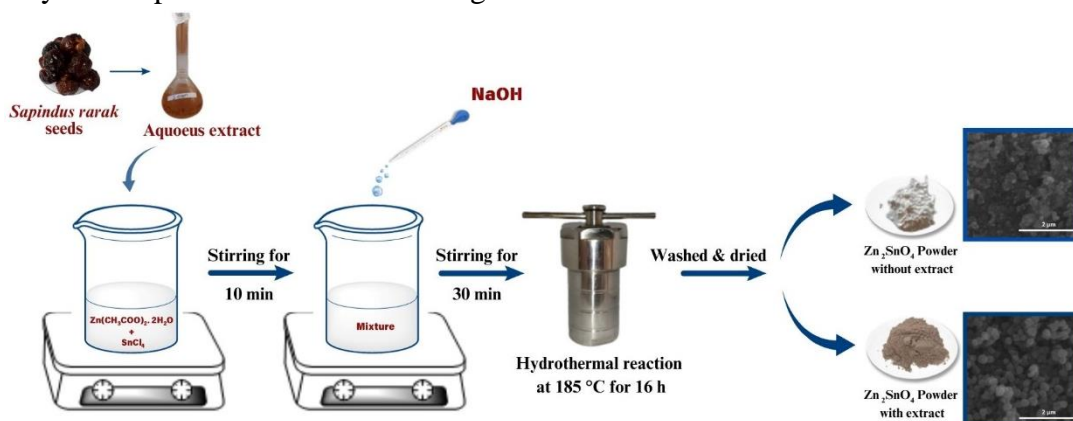
Figure 1. Schematic representation of the Zn 2 SnO 4 synthesis procedure using Sapindus rarak extract.
