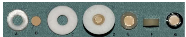
Figure 1. A. 5 mm x 1.5 mm standard Teflon mold for pulp capping material; B. Capping material obtained from the Teflon mold; C. 9 mm x 4 mm Teflon mold; D. Capping material and restorative material were placed into 9 mm x 4 mm Teflon molds. E and F standard samples of 5mm x 4 mm G. The restorative material which was placed onto capping material was closed with nail polish so that silver nitrate solution could penetrate from one place.
