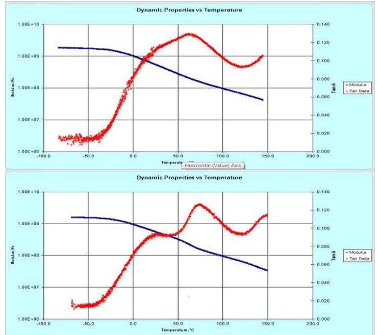
**Figure 7.** DMTA diagram of unmodified PU (Shore D) [Top] and PU (Shore D) PU 1% peroxide [Bottom].
