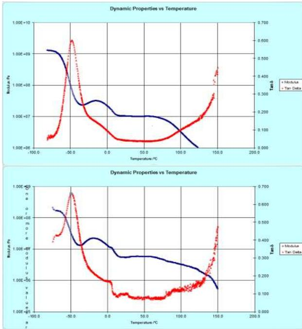
**Figure 6.** DMTA diagram of unmodified PU (Shore A) [Top] and PU (Shore A) 1% peroxide [Bottom].
