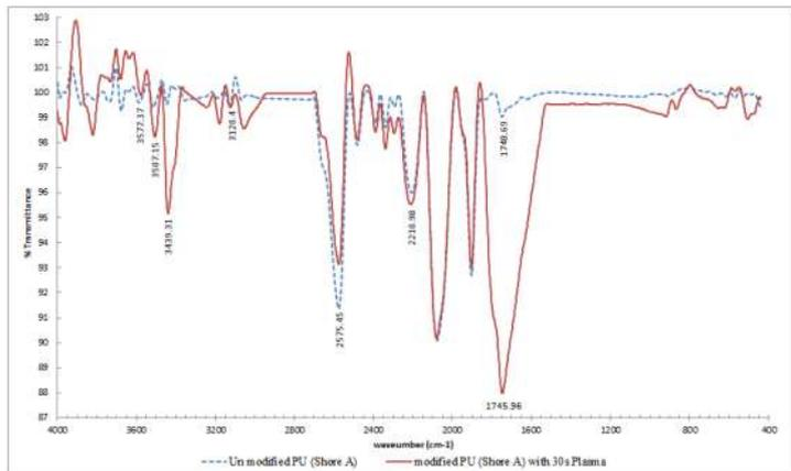
Figure 1. ATRFTIR spectrum of PU (Shore A) before and after 30s oxygen plasma treatment.
