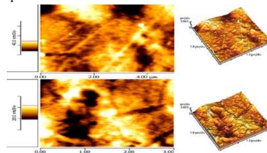
Figure 5. AFM images of plasma treated (Shore A) PU within 60s (Left) beside their 3D images (Right).
