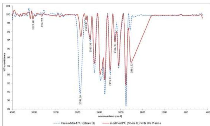
Figure 2. ATRFTIR spectrum of PU (Shore D) before and after 30s oxygen plasma treatment.
