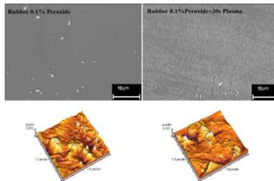
Figure 3. SEM and AFM images of unmodified PU (Shore A) and modified PU with 30s oxygen plasma treatment.
