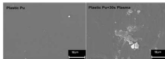
Figure 4. SEM images of unmodified PU (Shore D) and modified PU with 1% peroxide and 30s oxygen plasma treatment.
