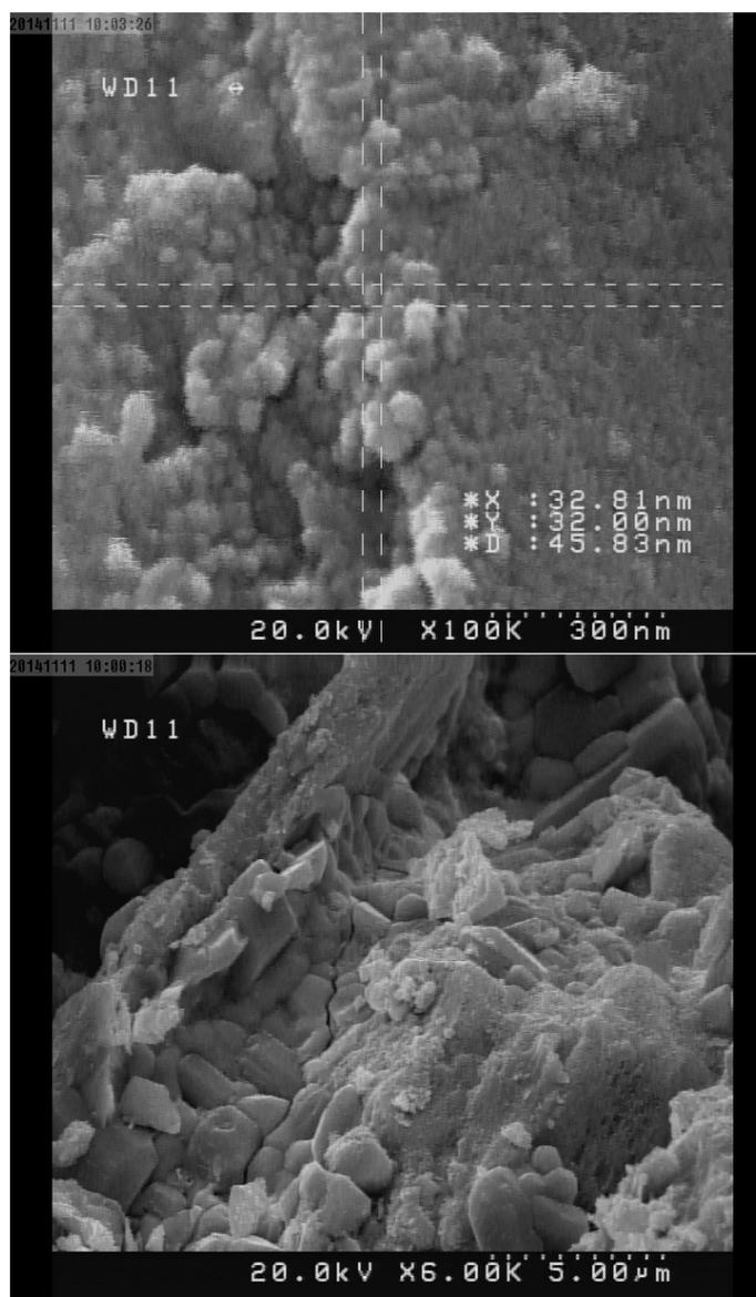
**Figure 2:** FE-SEM micrographs of Bi<sub>2</sub>O<sub>3</sub> nano-particles.
