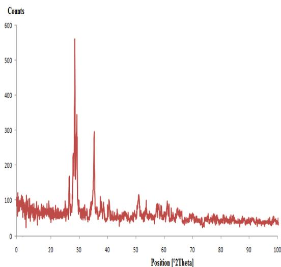
**Figure 1.** XRD pattern of Bi<sub>2</sub>O<sub>3</sub> nanopowder calcined in 600 °C.
