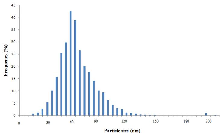
**Figure 3:** Particle size distribution of Bi<sub>2</sub>O<sub>3</sub> nanopowder.
