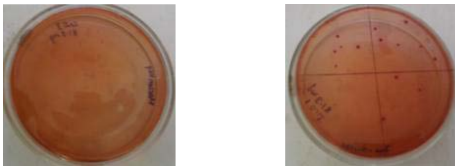
Figure 5. Bacteriocidal action of 1.0 mM \text{ZnO}_{1-x}\text{N}_x prepared by i) solution method and ii) equilibration method in MacConkey broth.
