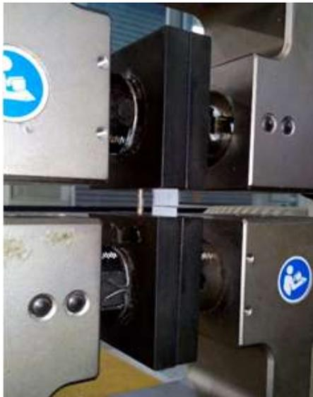
Figure 2. The single fiber was pulled in UTM for tensile testing.
