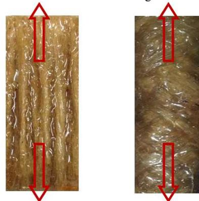
Figure 6. 90° and ±45° specimens of kenaf yarn fiber composite when Given Load (Direction of load).
