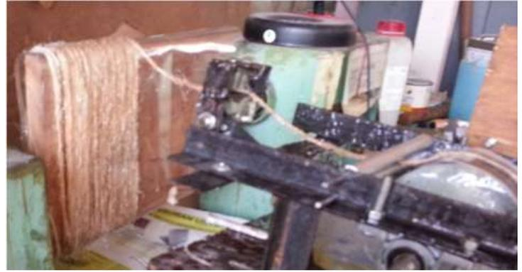
Figure 4. Filament winding of kenaf yarn fiber composite.
