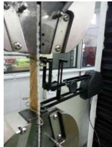
Figure 5. UTM, Instron 3382 for tensile testing of kenaf composite.
