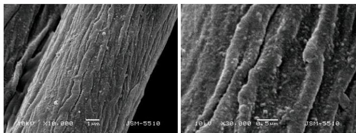
Figure 6. SEM micrographs of cotton fabrics treated with P1000-Napht with different amplification.
