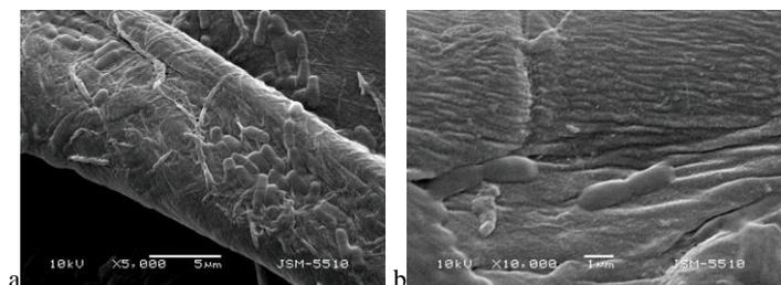
Figure 7. SEM images of cotton fabrics tested against *A. johnsonii* at magnification x5000 and x10000: a) biofilm on untreated cotton textile (control sample); b) the absence of biofilm on cotton textile treated with P1000-Napht.
