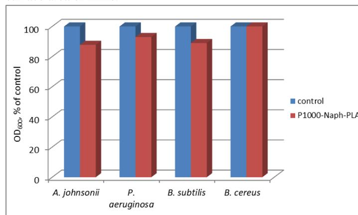
Figure 8. Effect of P1000-Napht-PLA film specimens on the growth of Gram-negative and Gram-positive bacteria tested in MPB.
