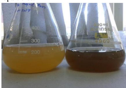
Figure 1. Control and Test flask showing color change due to bioreduction of silver nanoparticles.
