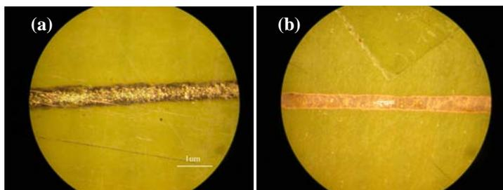
**Figure 6.** SNOM surface morphology of Cu deposited on the Ag by electro-less Plating. The adhesion of metal layer is: (a) f=10.18 Kg/cm<sup>2</sup>; (b) f=2.52 Kg/cm<sup>2</sup>;
