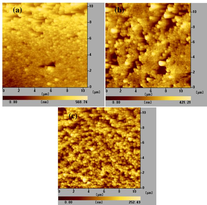
**Figure 7.** AFM surface morphology of the same substrate activated by different methods
