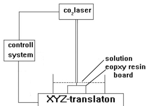
Figure 1. Setup for CO<sub>2</sub> laser-induced deposition from aqueous solution
