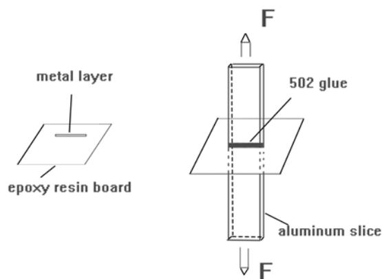
Figure 2. Measurement of adhesion of Cu layer with epoxy resin board
