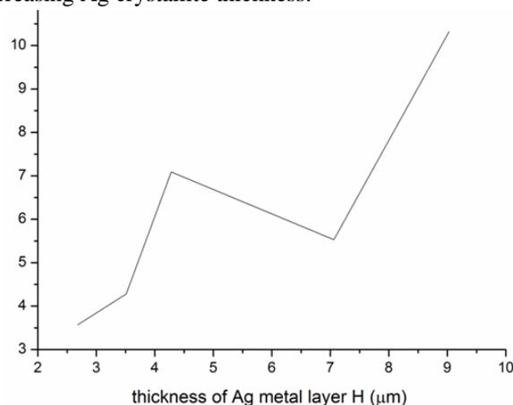
**Figure 4.** Curve of Cu layer adhesion and Ag crystallites thickness
