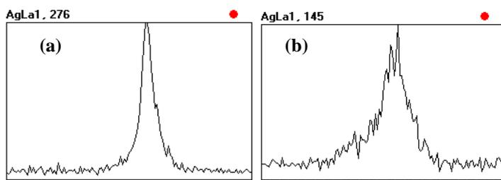
**Figure 3.** EPMA morphology of Ag crystallites of different thicknesses (line analysis); (a) laser power  $P=3\text{W}$  thickness: 5.5  $\mu\text{m}$ ; (b) laser power  $P=3.5\text{W}$  thickness: 9  $\mu\text{m}$ ;
