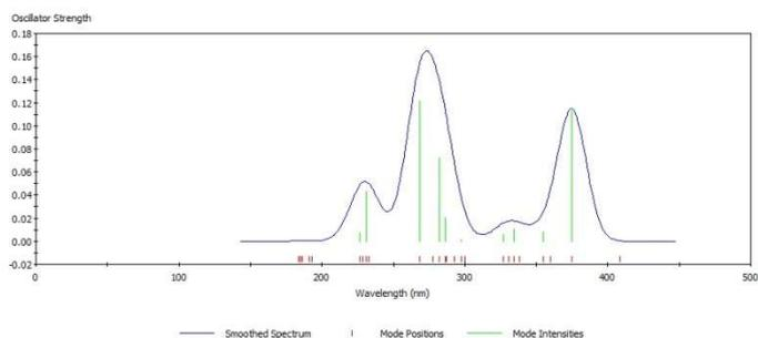
**Figure 4.** UV-Vis spectrum of FcSBCO molecule.
